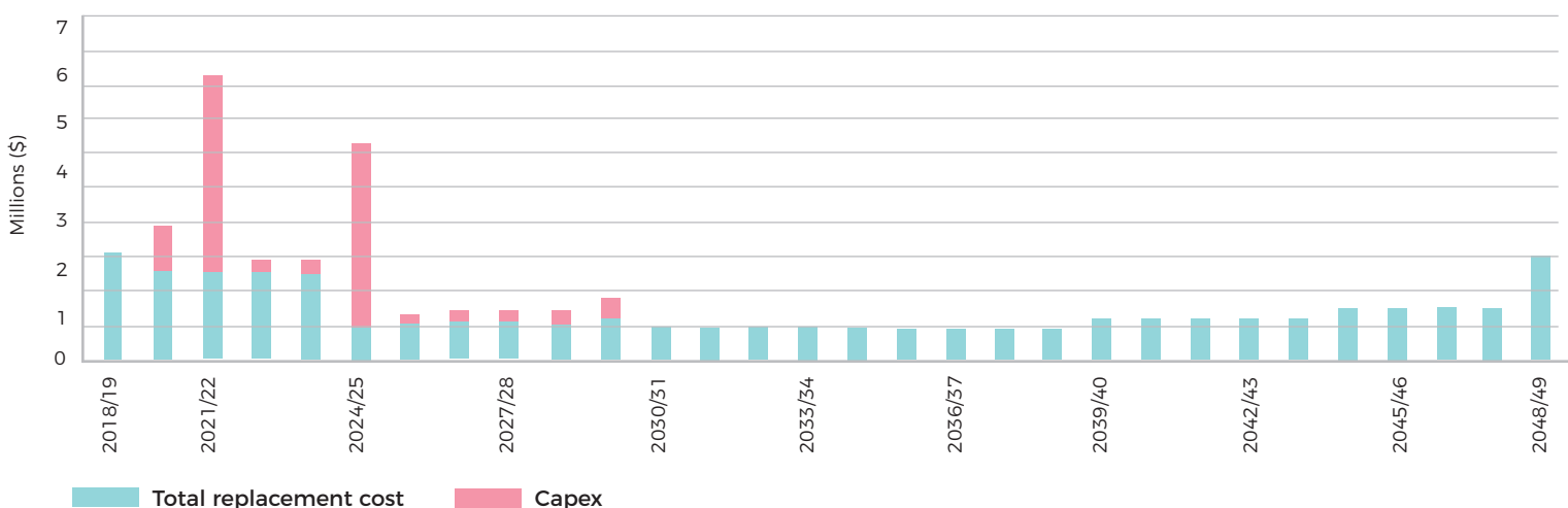
FIGURE 10 - WASTEWATER RETICULATION PROJECTED CAPITAL AND RENEWAL EXPENDITURE 2018-48 WASTEWATER PLANT CAPEX AND RENEWALS
