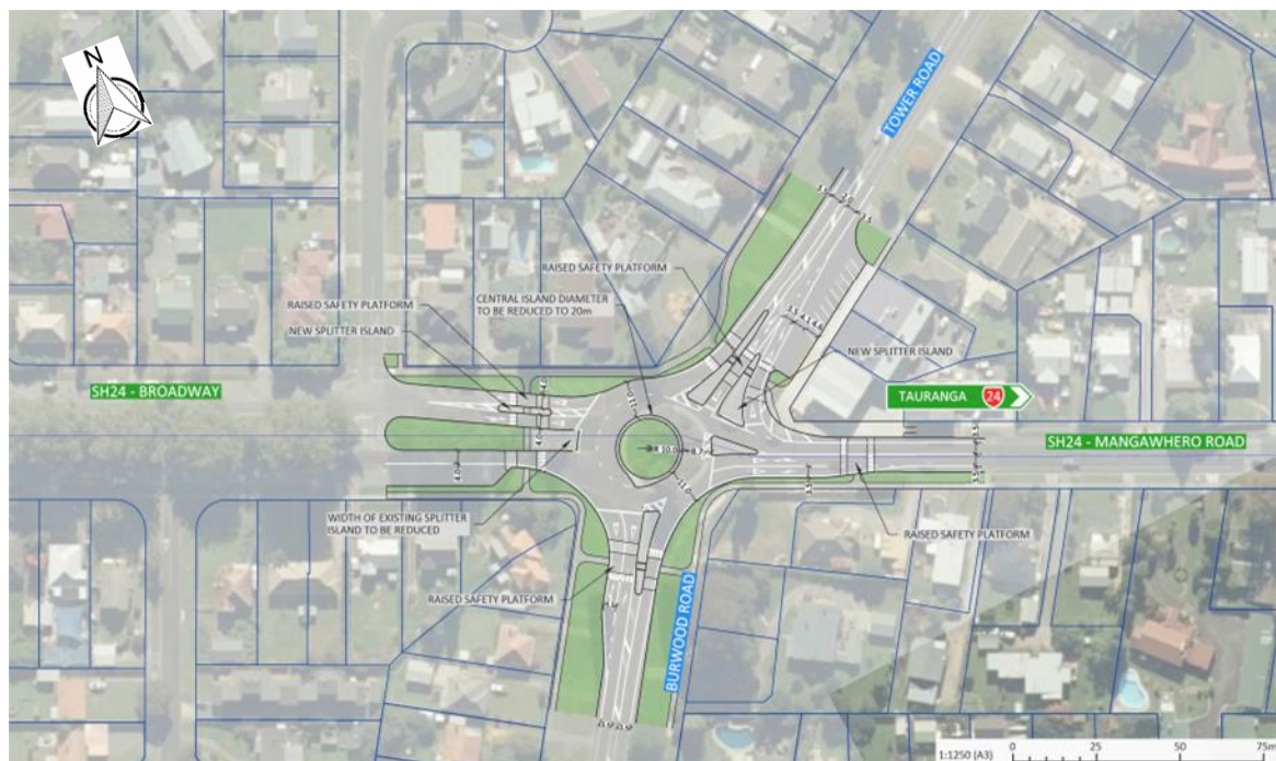
Figure 2: Proposed SH24/Tower Road/Burwood Road Roundabout Concept
